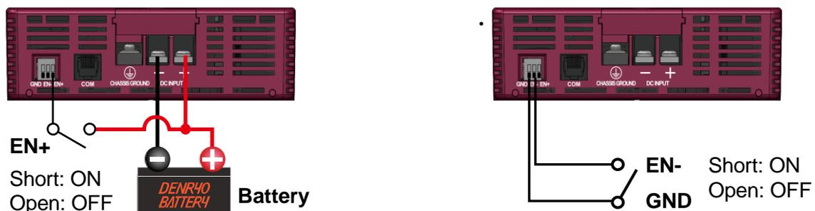
**Figure 5.4 The wiring of remote connector**
